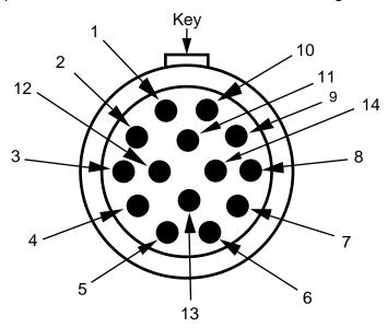
Pin numbering scheme for the cryocable connectors (LEMO receptacle), as seen when looking at the connector. The Key refers to the keyed slot on the warm end receptacle and the tab on the cold end connector.
