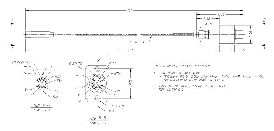
Mechanical specifications, Model CBL-C2-10 cryocable with 10-pin LEMO connectors. The standard length L is 1 meter.
