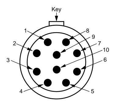
Pin numbering scheme for the cryocable connectors (LEMO receptacle), as seen when looking at the connector. The Key refers to the keyed slot on the warm end receptacle and the tab on the cold end connector.
